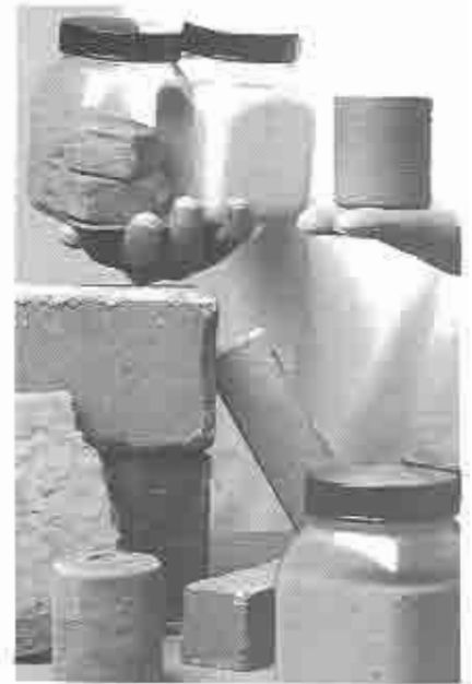
The most hazardous components can be stabilised by solidification.
