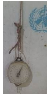
The balance used to weigh the waste before burning
