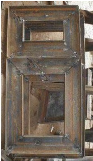
Fig. 6. the top frame with U shaped to be filled with white construction sand.
