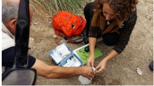
Picture 2 : Field Testing of Free Chlorine Residual
