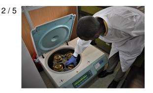
Laboratory technician Benlick Mwangi unpacks the centrifuge used to spin environmental samples to separate any polioviruses that might be present from any sludge in the sample. Environmental surveillance for polioviruses is used to detect polio in a large catchment area before it causes paralysis in children.
