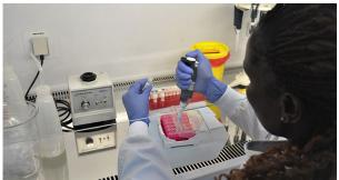
Laboratory technologist Agnes Chepkurui prepares samples for the final stage of testing for polioviruses within the laboratory. This stage of the process is conducted if suspected polioviruses are identified in the cell culture under a microscope, in order to find out what kind of virus it is. WHO/L.Dore
